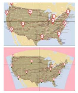
Figure 6. Reprojecting from a conic projection requires bending straight lines.
